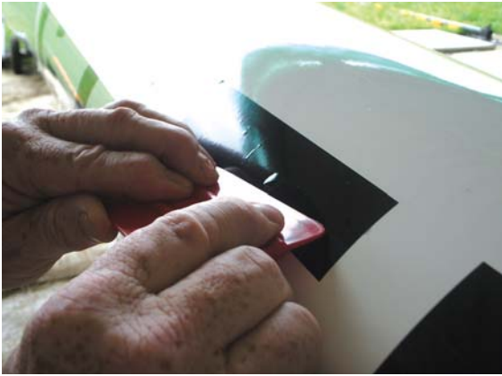
Easing out bubbles to edge with squeegee
