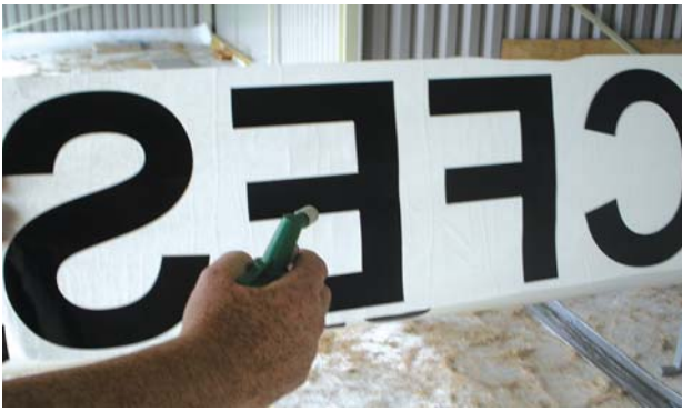
Lightly spraying adhesive side of vinyl whilst holding taut
